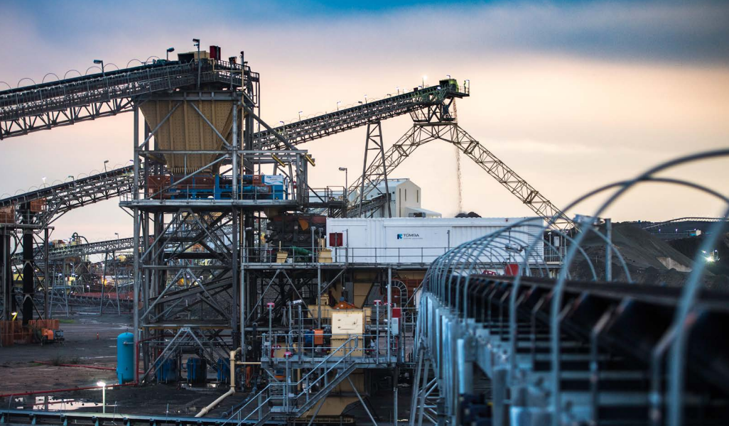
Mega Diamond XRT (X-ray transmission) facility or MDR (mega diamond recovery) unit
