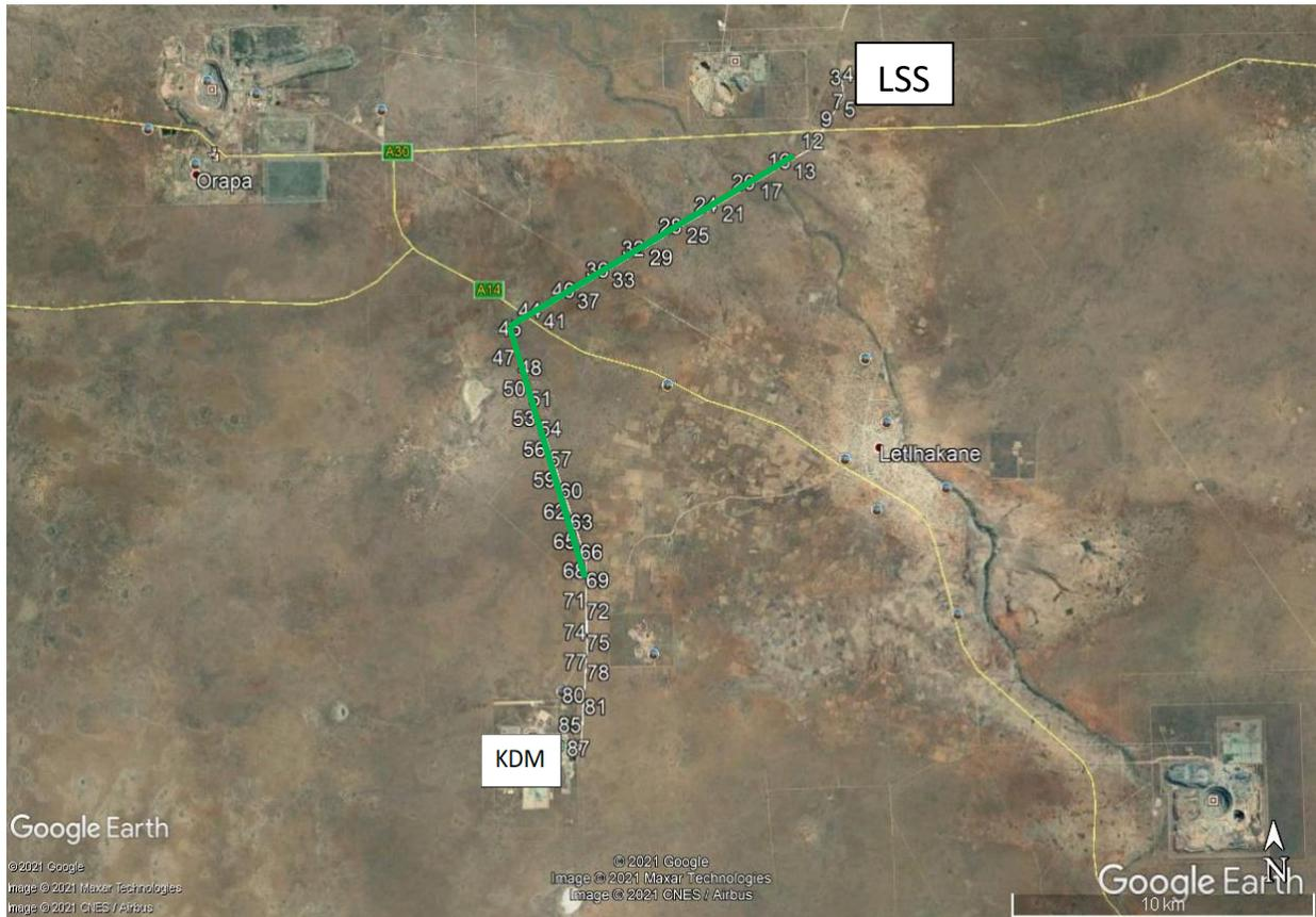
Note: KDM – Karowe Diamond Mine, LSS – Letlhakane Substation; Transmission lines section marked in green part of designated areas for bird mitigation (deflectors). Source: Lucara and contractors.
