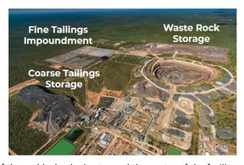
designed to maximize water capture with each of the paddocks sloping toward the centre of the facility. This allows for recycling of water to be used in the process plant.
